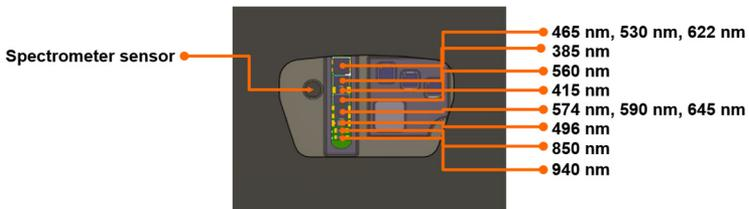
Figure 21: Positions of excitation LEDs for illumination of the shake flask and the spectrometer sensor for fluorescence measurement on the MPS. The top of the image is oriented towards the shake flask wall, the bottom towards the center of the flask.
