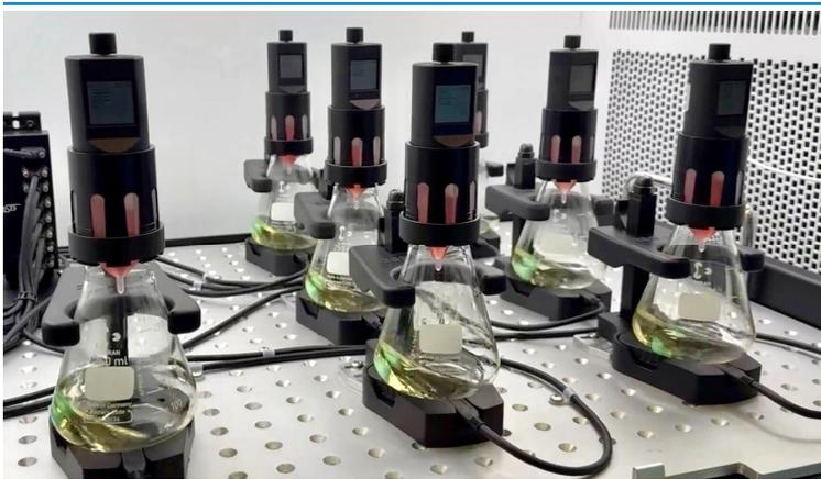
Figure 2: The Multiparameter Sensor combined with the LIS Feeding system. The online parameters biomass, fluorescence, and DO can be utilized to trigger and control feeding.
