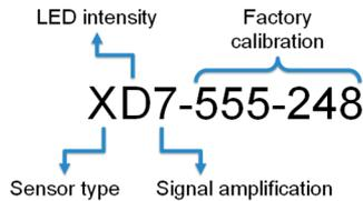
**Figure 24:** Types of information in the DO Sensor Code. The first three digits specify the detection settings, which are: Sensor Type: X = DO Sensor Pill; LED intensity: A-H (A = lowest, H = highest); Signal amplification: 1-7 (1 = lowest, 7 = highest). The center and last three digits contain the factory calibration that converts the raw signal to dissolved oxygen data (DO partial pressure; DO Percent (air saturation)).
