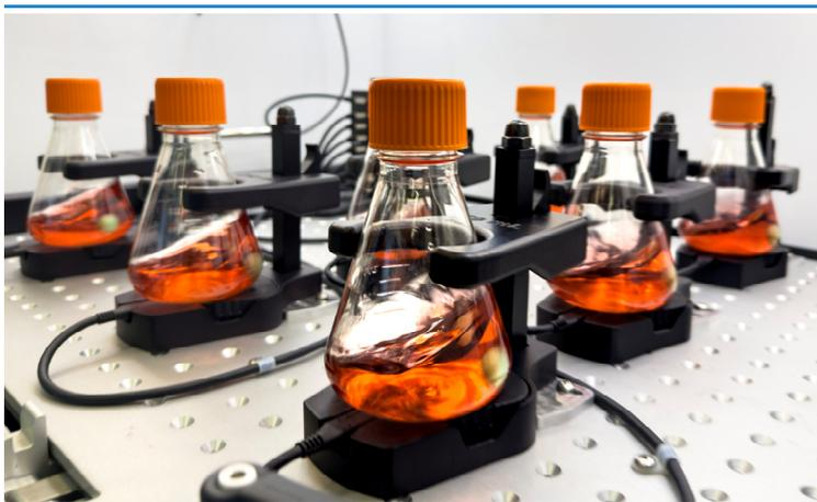
Figure 1: Multiparameter Sensors monitoring biomass, fluorescence, and DO via DO Sensor Pills in a cell culture application.
