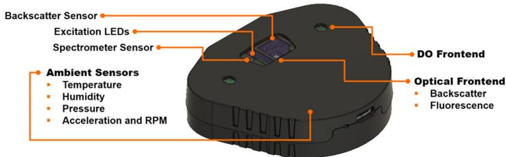
Figure 3: The MPS combines backscatter, spectrometer, DO and ambient sensors into one single device.
