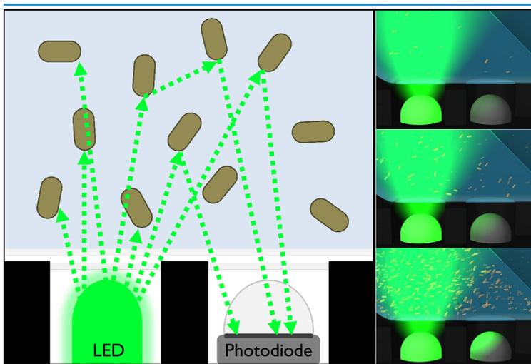
Figure 19: Optical cell density measurement using light scattering.
