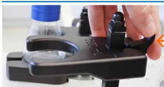
Lower the handle on the back of the Adapter ring to lift the ring upwards.
