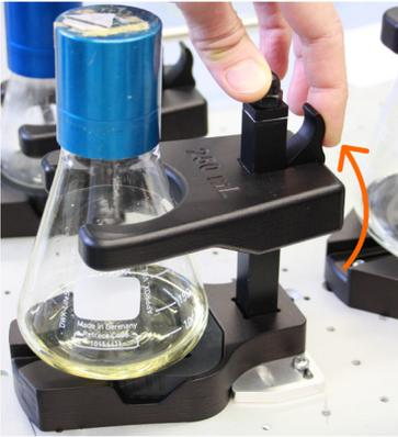
Push the handle completely up to fix the ring in place.
