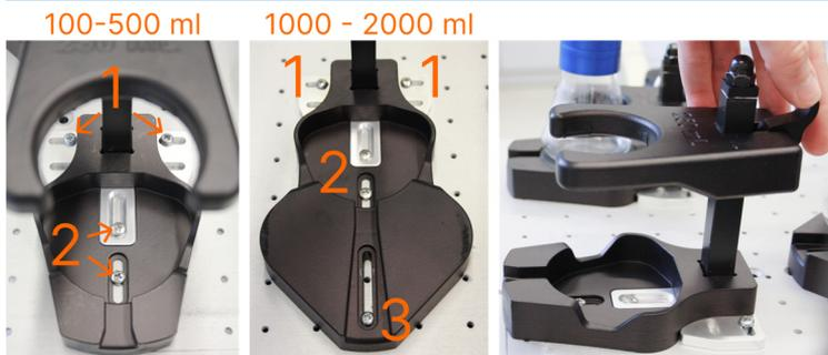
Figure 8: Shake Flask Adapter 250 ml (left) and 2000 ml (center) screwed into a shaking tray (1 – screws on the back plate, 2 – screws in base center, 3 – additional screw on large Adapters). The handle on the back of the Adapter ring (right) is lowered to slide the ring up or down.
