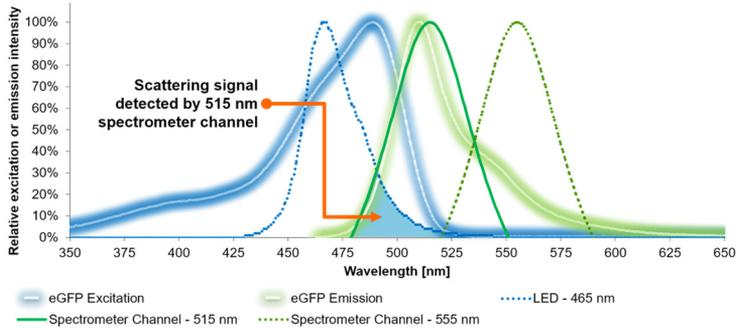
**Figure 22: Exemplary guideline to select excitation and emission configurations of the MPS for eGFP<sup>1</sup>.** A combination of the 465 nm LED with the 555 nm spectrometer channel provides sufficient eGFP excitation and emission spectra coverage while preventing scattering interference due to overlapping LED and spectrometer channel spectra.
