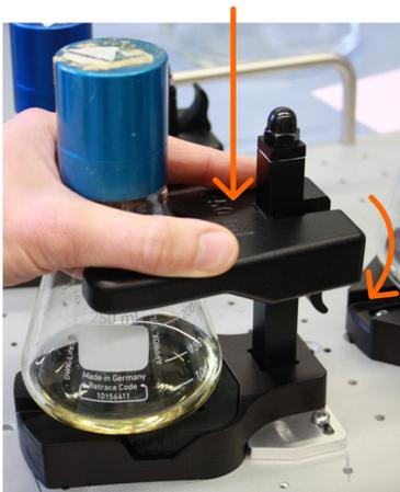
With the handle kept down, move the Adapter ring down until it embraces the shake flask.
