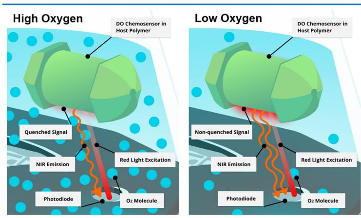
Figure 23: Working principle of the DO Sensor Pills.
