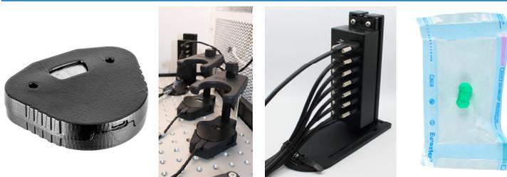
**Figure 7:** Components of the multiparameter sensing system: The MPS (Multiparameter Sensor), the Shake Flask Adapter holding the MPS with USB cable, the MPS Hub (7 MPS ports), and the single-use DO Sensor Pill.
