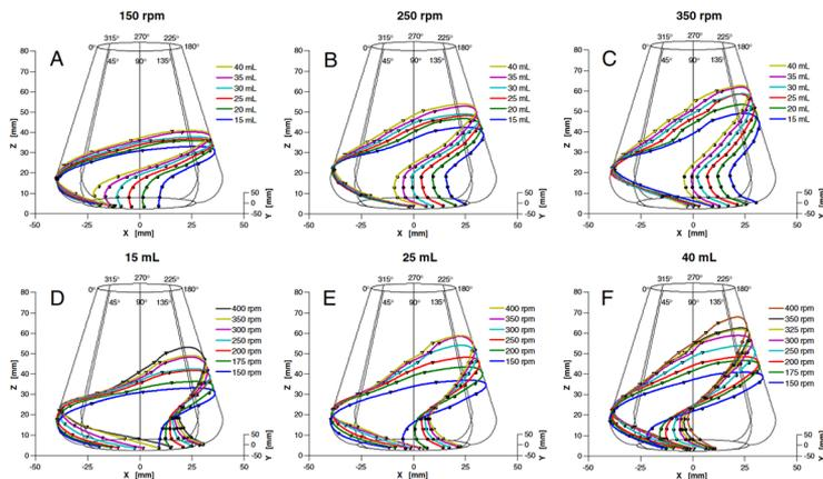
Figure 25: Illustration of the 3D-distribution of the bulk liquid under different shaking and filling conditions in a 250 ml non-baffled flask.<sup>3</sup>
