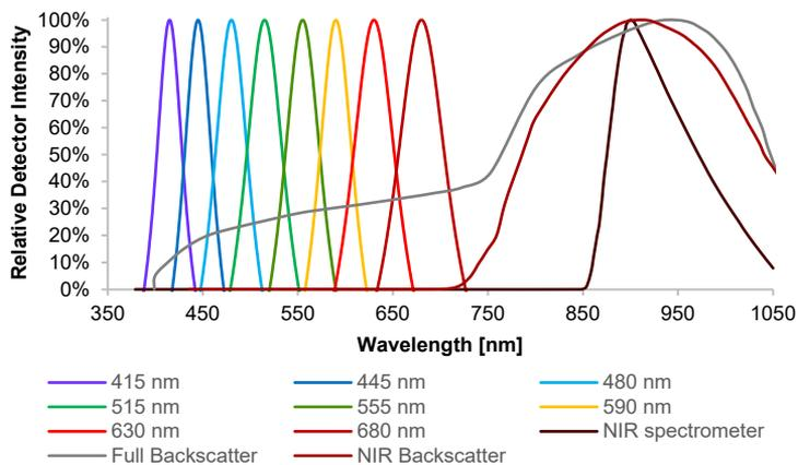
Figure 6: Detection spectra available on the MPS. The intensity scale is relative to each peak maximum.
