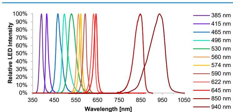
Figure 5: Spectra of LEDs used for backscatter and fluorescence monitoring. The intensity scale is relative to each peak maximum.
