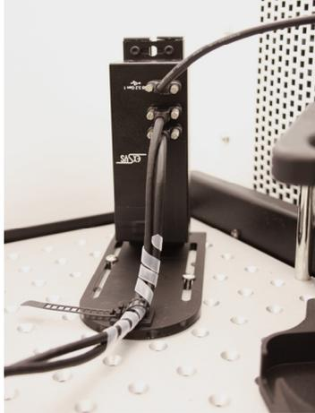
Figure 9: MPS Hub installed on the shaking tray. The topmost USB-C port is used to connect the Hub to the computer. The ports below connect the MPS devices to the Hub (in this case, 2 MPS).
