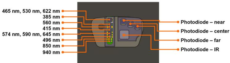
Figure 20: Positions of LEDs for illumination of the shake flask and photodiodes for backscatter measurement on the MPS. The top of the image is oriented towards the shake flask wall, the bottom towards the center of the flask.
