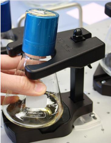
Place the shake flask onto the MPS, with the shake flask neck located inside the Adapter ring.
