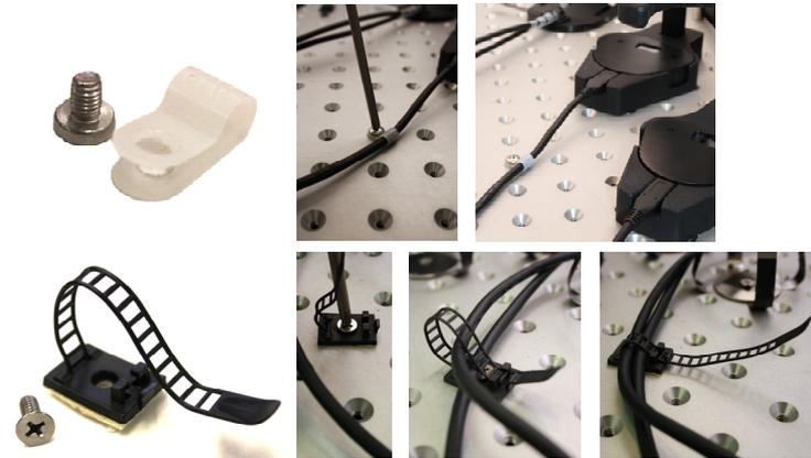
Figure 12: Single (top) and multi-cable (bottom) management tools for fixing cables onto the shaking tray.
