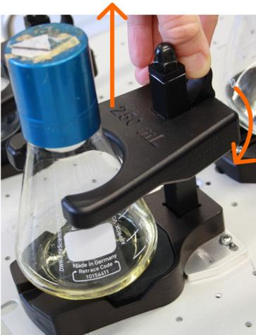
Lower the handle on the back of the Adapter ring and lift the ring upwards until it is possible to remove the flask. In some cases, the flask neck might slightly stick to the Adapter ring, be careful and hold onto the flask while moving the ring upwards.
