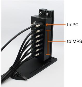
Connect a USB-cable from the USB-Hub to each MPS. Any port can be used for an MPS as long as the topmost port is correctly connected to the computer with DOTS Software.
