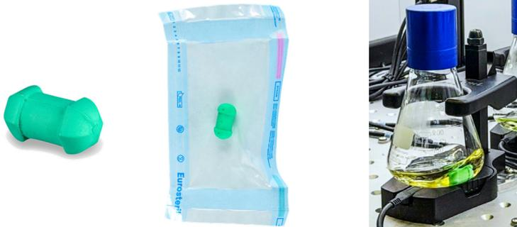
Figure 4: The Sensor Pills - DO come individually sterile packaged and are added directly into the shake flask.
