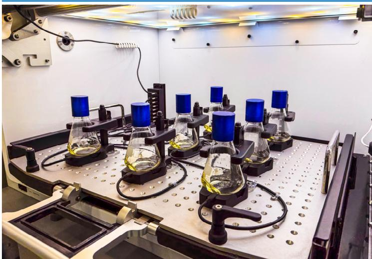
Figure 14: Cable management inside the shaker.
