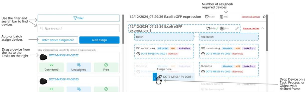
Figure 61: Experiment Creation wizard – Device Assignment: Drag and Drop
