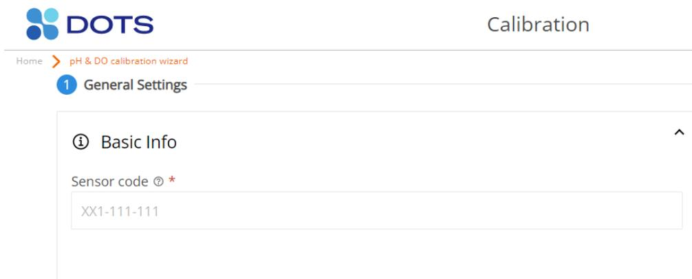
Figure 106: Enter the correct Sensor code for either a pH or DO flow cell, depending on the type of calibration you would like to perform
