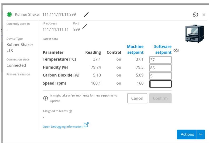
Figure 50: Smart Shaker direct controls in the Device Details.
