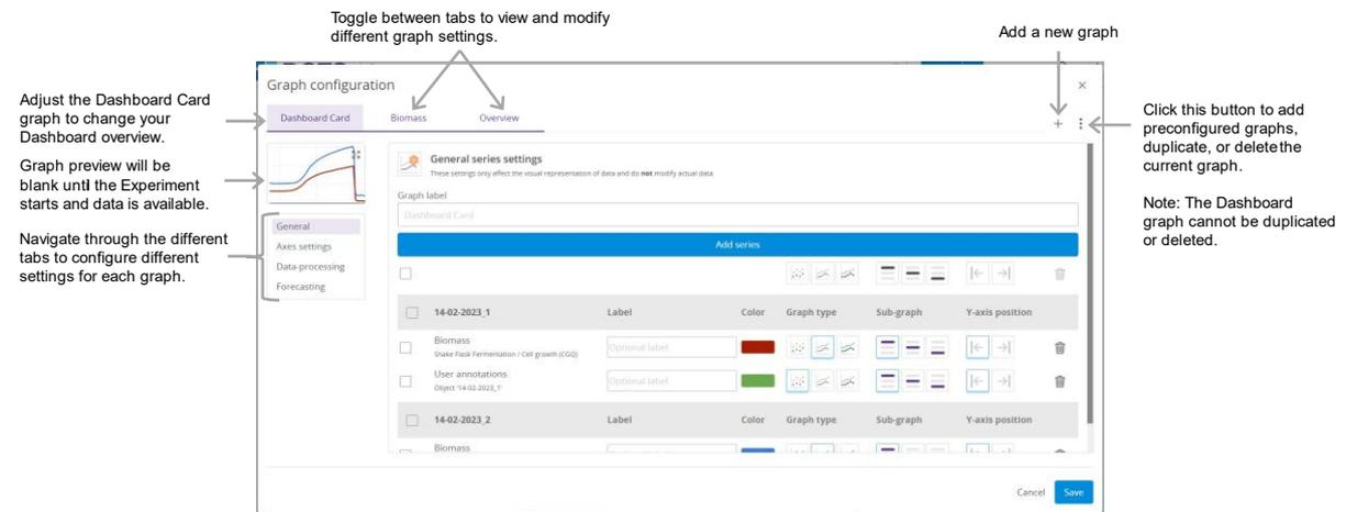
Figure 82: Graph configuration window – General tab
