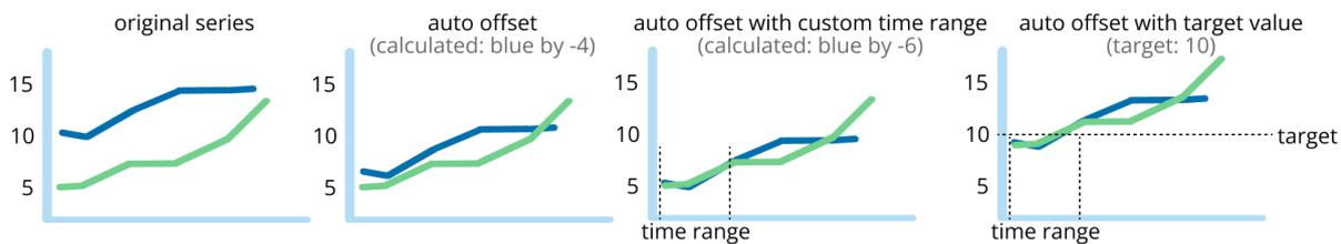
**Figure 85: Applying automatic y-axis offsets with different control options**
