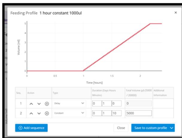
Figure 93: Editing a LIS parameter set (left) and defining a LIS Feeding profile (right).
