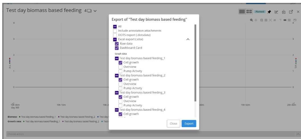
Figure 90: Dashboard data export pop out – expanded view. Customize which data is exported by checking the boxes next to series of interest.
