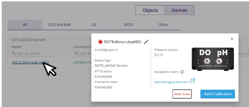
Figure 105: The pH & DO Calibration wizard is accessible via the DOTS Fiber Optic Sensor Device Details pop out
