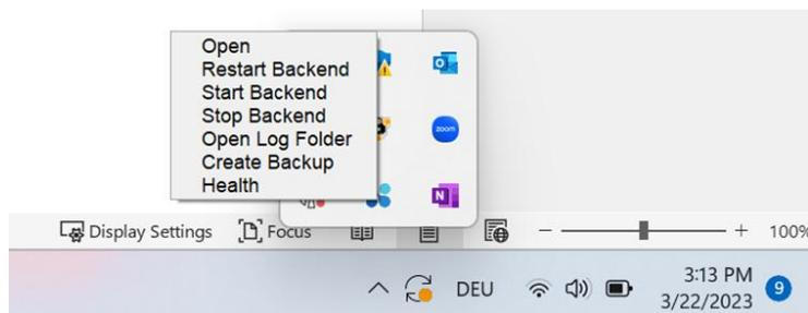
Figure 118: Options available via the DOTS system tray icon
