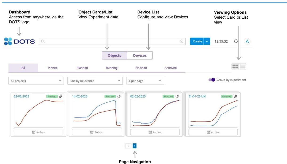
Figure 41: The DOTS Software Dashboard – an overview
