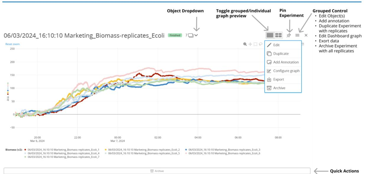
Figure 43: Grouped graph pop out. By default, the primary data series for all Objects in an Experiment group are shown.
