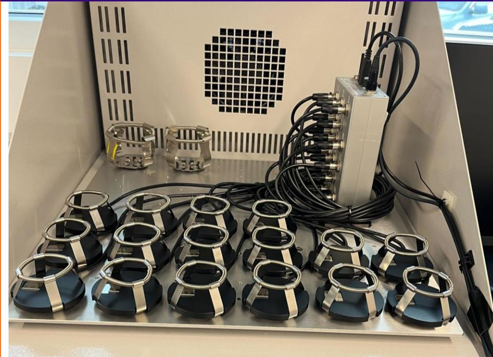
Guide the cables using the cable clamp array.
